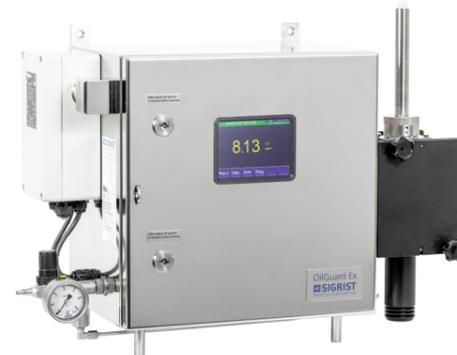
Ex OilGuard with a pressurized enclosure system
